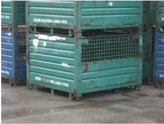
FORD ZE-13 SOLID CONTAINER 53" X 48" X 40" HIGH SOLID SIDES & FLOOR / MESH DROPGATE FORK STIRRUPS & PIN FEET $219.00 EA
